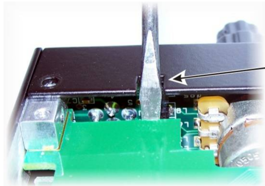
Figure 9. Separating the Front Panel Assembly from the Chassis.
