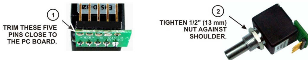
Figure 17. Checking and Trimming the VFO B Encoder Pins.
