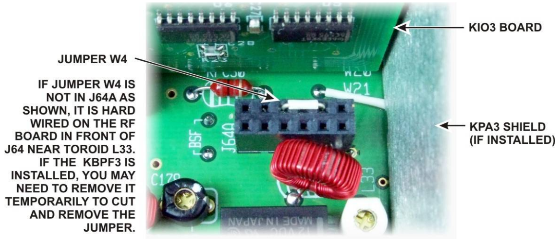
Figure 45. Jumper W4 on the K3 RF Board.
