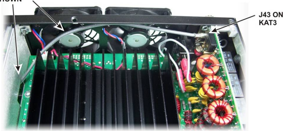
Figure 29. Optional KRX3A Antenna TMP Cable to KAT3.
